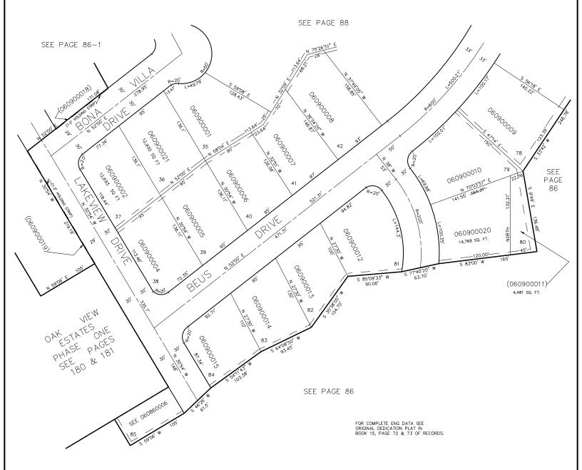
5' UTILITY & DRAINAGE EASEMENTS EACH SIDE OF PROPERTY LINES AS INDICATED BY DASHED LINES EXCEPT AS OTHERWISE SHOWN.
